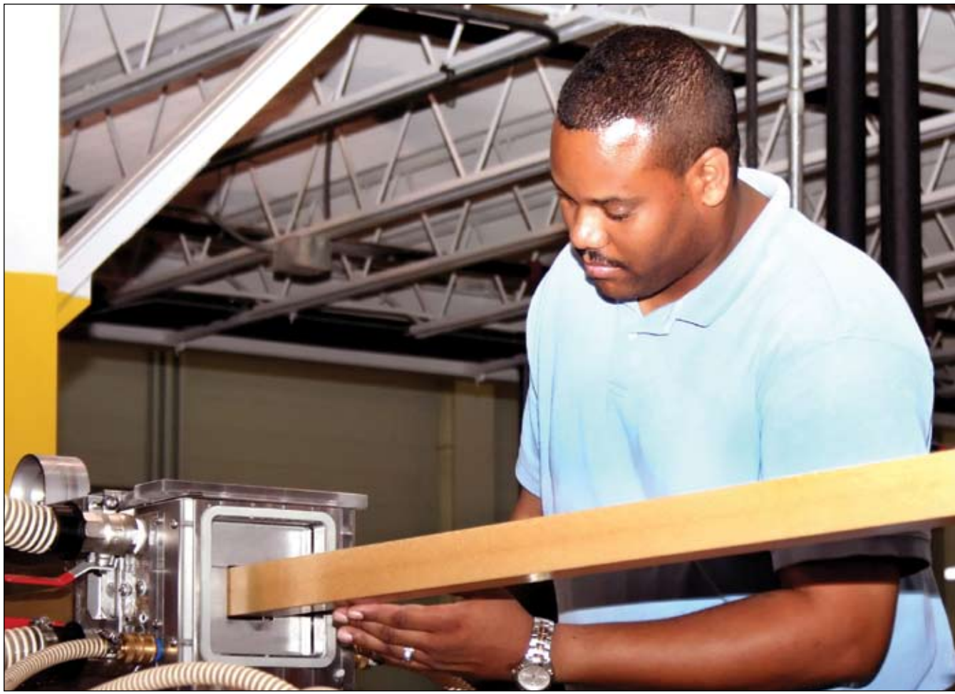
Staff photos by T.M. James Kelvin Wright checks a piece of decking rail Wednesday on an extrusion machine at the Tech-Wood facility in Greenwood.
